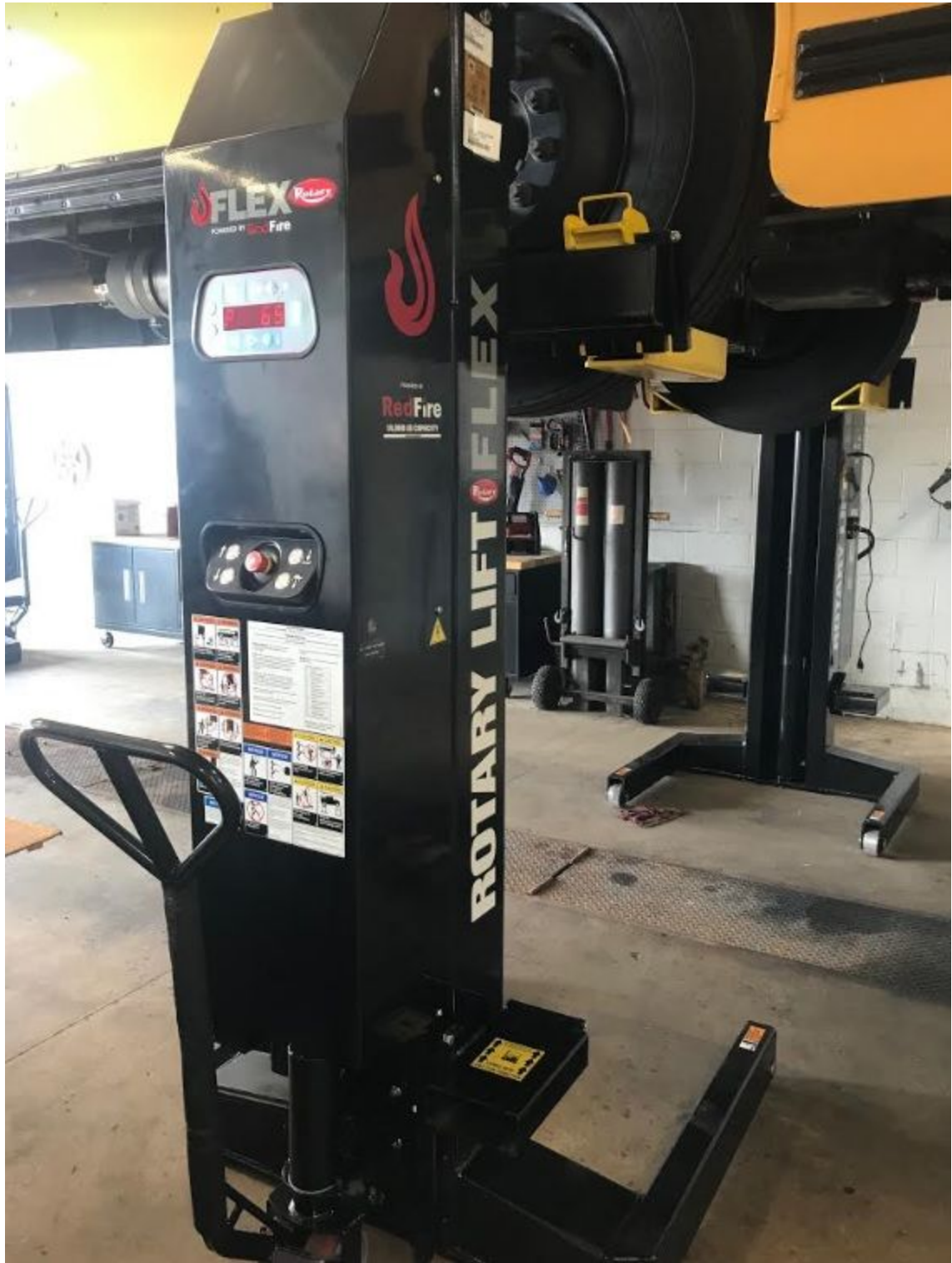
Pictured below: A side view of one of the four posts from the new four-post vehicle lift.
