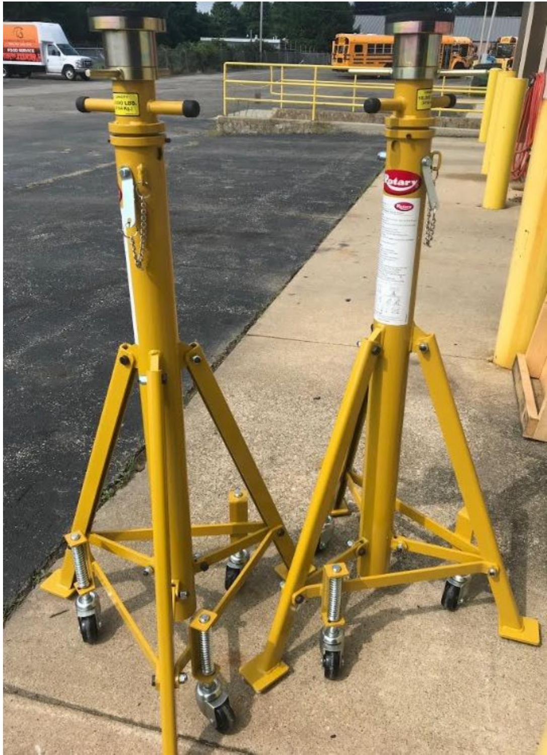
Pictured below: Two of the four new jack stands (rated for 18,000 lbs each).
